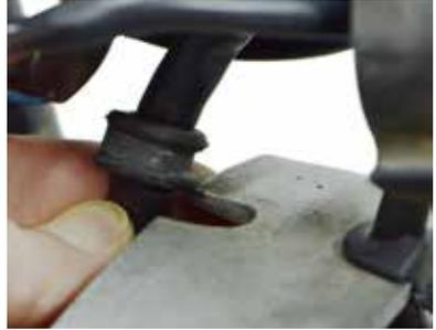
Once you free the grommet from the top of the engine cover, follow the wires up to the voltage regulator. Unplug the 3 pin connector from the voltage regulator and remove it, replacing the screws back into the frame.
