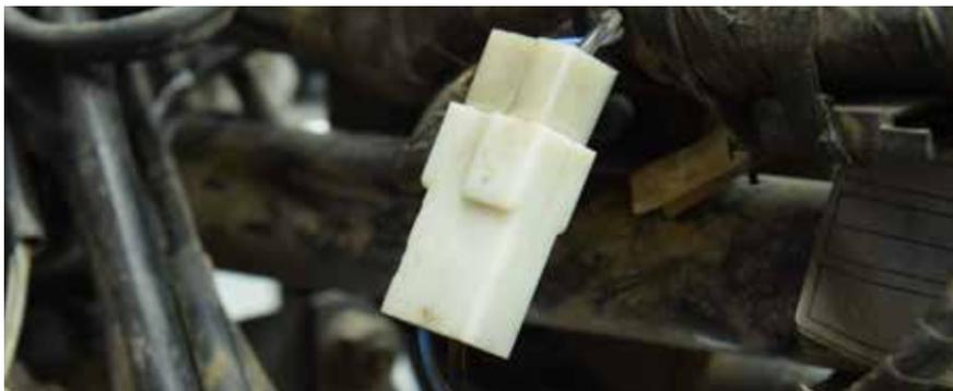
This connector can be problematic to disconnect. Take care when working with plastic connectors that are aged and brittle.
