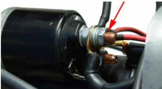
You will need to make a wire to connect the double red wire from the chassis harness to battery voltage. *It will match HAR-4B however needs a male spade terminal instead of female.* This wire runs from the **starter solenoid positive terminal**, to the **double red wire** from the chassis harness. This wire supplies voltage to power the bike.
