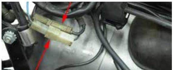
The **BLUE** wire from **HAR-4A** goes to the **BLUE** wire in the white plug. You will have to change this terminal from a Female to a Male terminal on the HAR-4A with the terminal provided in the kit. This wire is connected to the generator light in the instrument cluster.
