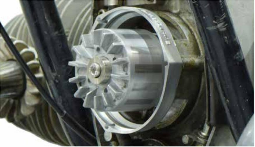
Fit the stator and outer ring. Take note of the cutouts on the stator body to allow the mounting bolts to pass through. Note the stator wires are approximately in the 6:00 position.
