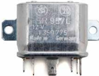
Unfortunately now the starter relay has no way of knowing if the vehicle is running, and will not start the bike. To restore the starter relay function to the bike, a new starter relay needs to be wired in. In doing so remember, the safety feature of starter lock out will be removed! This modification should not be taken lightly as your safety is paramount to our company and your loved one's.
