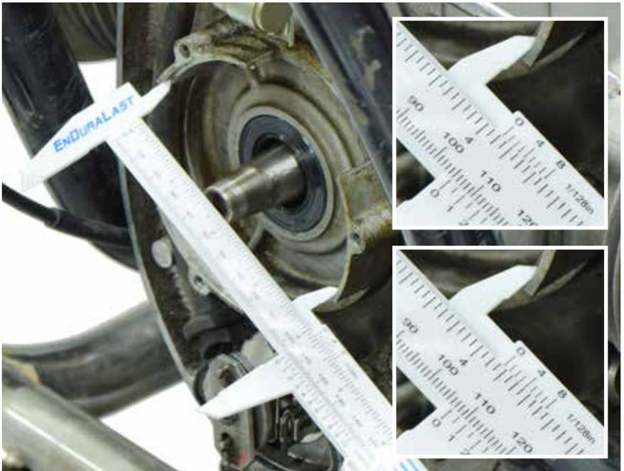
The seating of the inner stator frame into the timing chain cover machined groove is precise and tight! If there is ANY side to side movement or play in fitment, then you have selected the wrong inner ring.
