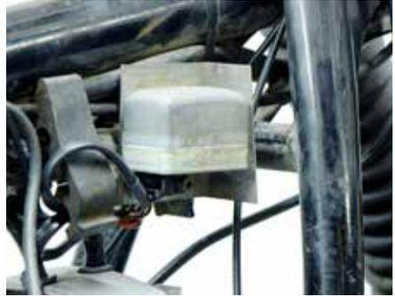
A mounting bracket is included that will allow you to mount the R/R in the original location. Assemble as illustrated below. It is tricky to secure everything in such a tight area, the use of a needle nose pliers is recommended.
