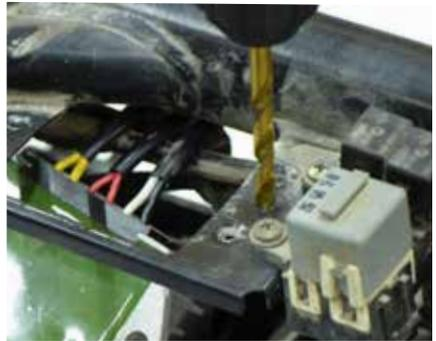
Mount the R/R to the underside of the bracket with the included hardware. Note the R/R case is its ground connection, and for it to function properly and for its longevity, a solid ground connection is required. You may find it advantageous to install the additional ground strap included to ensure a proper ground connection.
