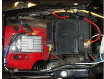
Note when you are mounting the R/R, the case is its ground connection, so if you mount it on rubber bumpers for example, you will want to use the included ground wire. A poor ground connection can cause premature failure of the R/R. It is always a good idea to add your own additional ground strap to ensure the systems longevity.
