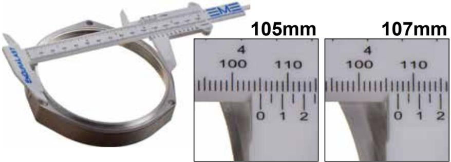
Measure the groove on the engine where the inner stator frame fits to determine which inner ring to install.
