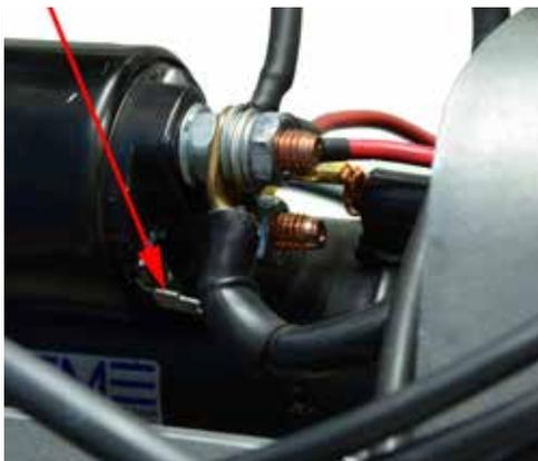
Install **HAR-4C** between the starter relay terminal **G** to the starter **solenoid spade terminal**. This is what will trigger your starter to engage when you press your starter button.
