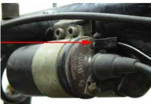
Run **HAR-4D** from the ignition **condenser** to the **coil negative** (terminal #1). This replaces the original ignition wire removed with the front engine harness.
