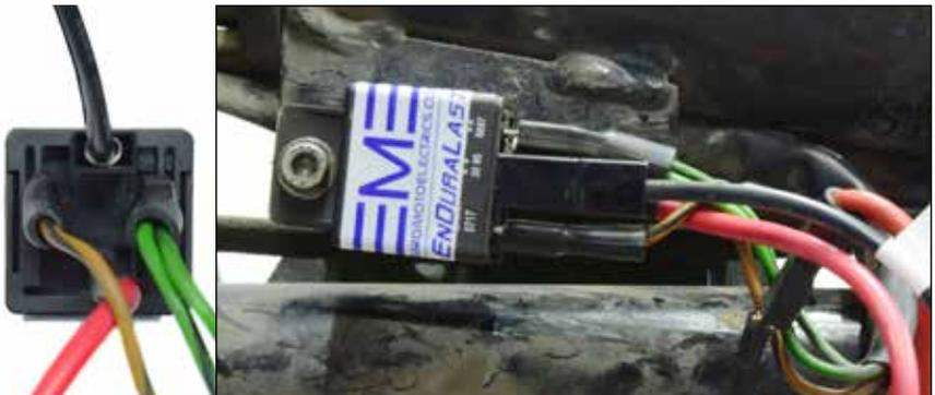
The relay will now look like this and can be secured with one of the original relay mounting screws to the frame as shown.
