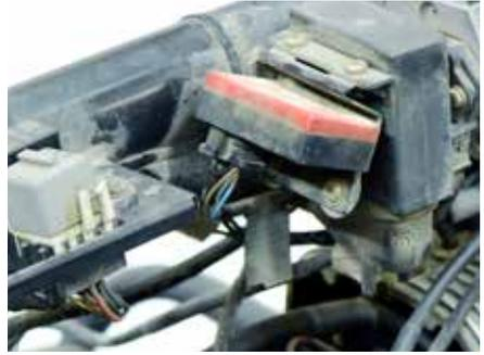
For these models, further back on the center frame is a reasonable location to mount the R/R as shown. Start by relocating the relays to the opposite side of the mounting bracket to clear room for the R/R. Drill out the existing screw hole to the rear to accept the mounting bolt.
