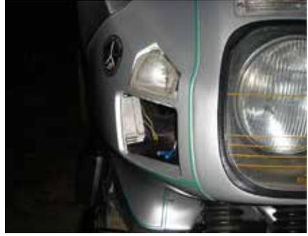
In some custom applications it is mounted on the front of the bike where you would often find a horn. This location is great as it will receive ample cooling and air flow.
