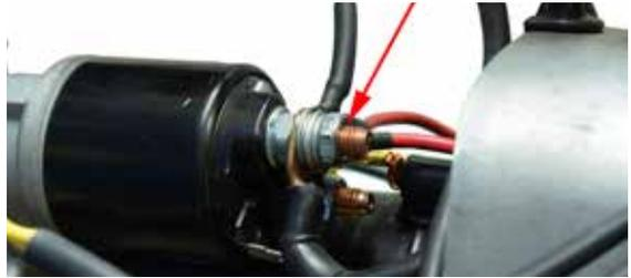
Connect the **BLUE** wire to the **BLUE** wire previously connected to the starter relay, coming out of the main chassis harness. This wire is connected to the generator light in the headlight.
