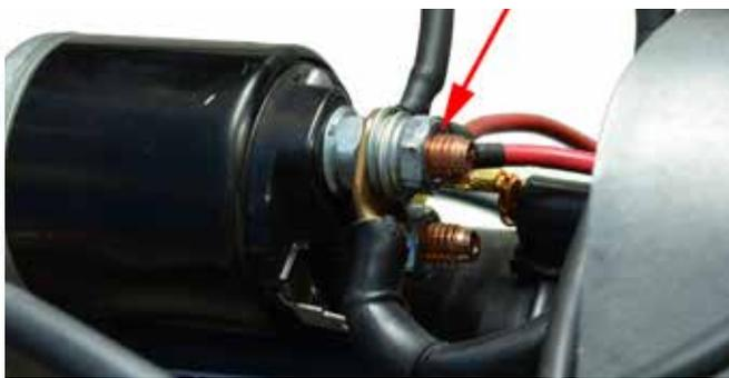
Run **HAR-4B** from the new starter relay terminal **30** to the **starter solenoid positive terminal**. This will provide power to the starter relay.
