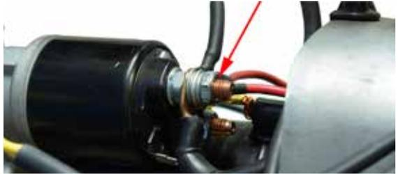
Connect the **BLACK** wire (with piggyback terminal) to the **coil positive** terminal. Use the piggyback to reconnect any wire (typically **GREEN**) that was removed to make this connection if needed. *Stock coils should have open terminals.*
