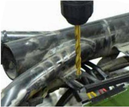
Measure forward 92mm on center and drill the second hole.
