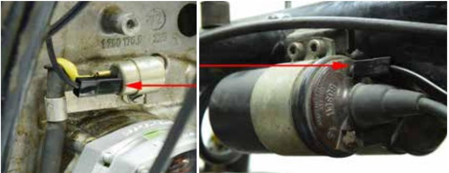
Run **HAR-4D** from the ignition **condenser** to the **coil negative** (terminal #1). This replaces the ignition wire removed that was part of the front engine harness.
