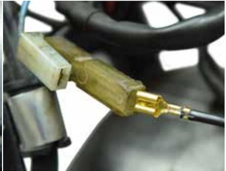
Run **HAR-4E** from the **Starter Solenoid Spade Terminal** to the **BLACK** wire in the white plug as shown. If your model does *not* have this plug, you will replace it with the bare connector into the relay block replacing the trigger wire for the starter. This wire will trigger the starter when the start button is pressed and replaces the original wire when you removed the engine harness.
