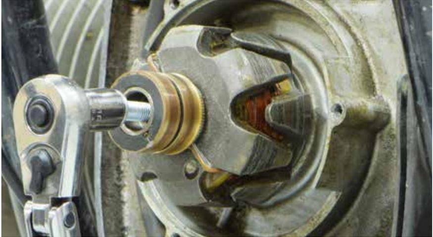
Gently tapping the rotor with a rubber mallet after tightening the removal tool can assist in releasing the rotor from the crankshaft. The rotor can “pop” off the end of the crankshaft, so be prepared! You may need to put the transmission in gear to keep the engine from turning over during this process.
