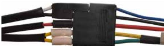
Connect the **WHITE PLUG** with yellow / green wires to the **WHITE PLUG** from the stator.
