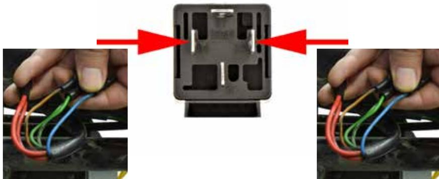
Connect the main harness **BROWN** to **86** and **GREEN** to **85** on the replacement relay.
