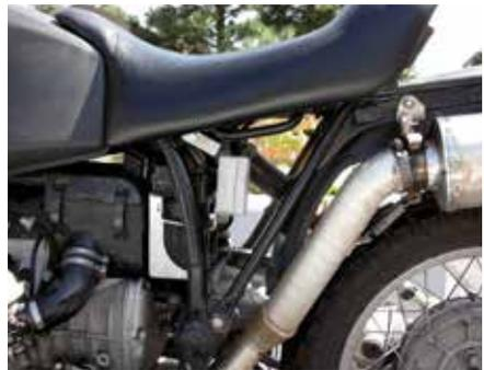
One location that is **NOT** recommended is **UNDER** the front engine cover, where the original diode board is located. Per the manufacturer (Ducati Energia) this R/R is not to exceed 194°F/ 90°C. The operating temperature here has been measured at 215°F/ 102°C. Do not cut or modify the R/R housing as it will more than likely cause damage.
