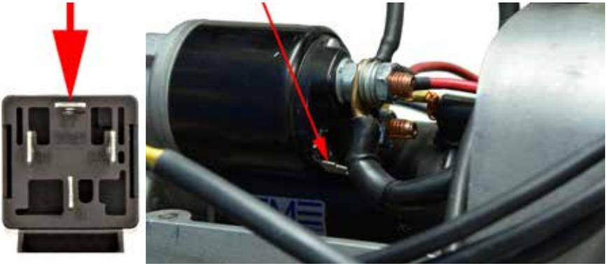
Run **HAR-4C** from the **starter solenoid spade terminal** to the new starter relay terminal **87**. This will trigger your starter to engage when you press your starter button.
