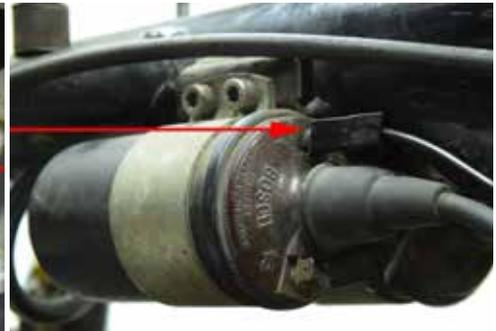
Run **HAR-4D** from the ignition **condenser** to the **coil negative** (terminal #1). This replaces the original ignition wire when you removed the front engine harness.
