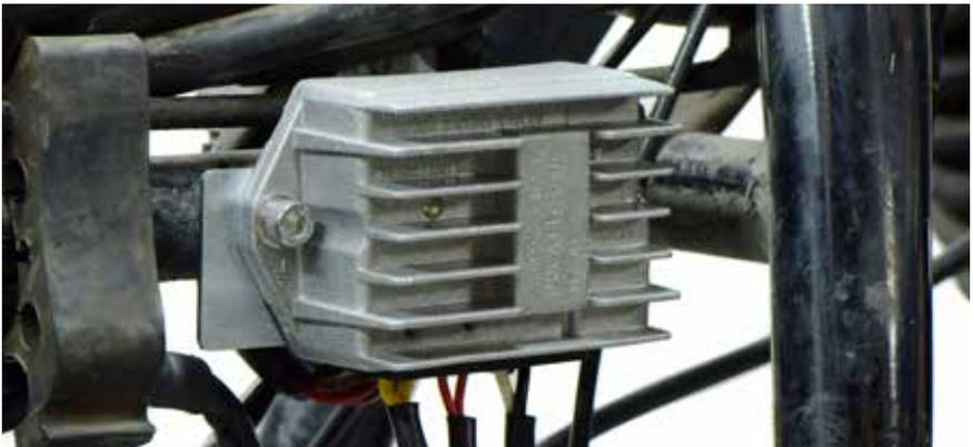
**Later BMW models** have the voltage regulator mounted as shown here.
