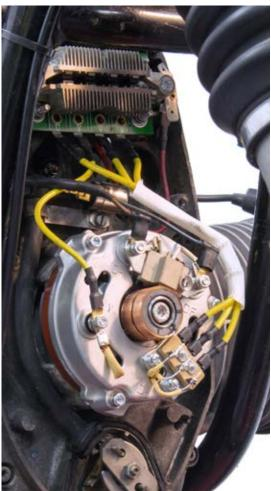
The short yellow wire included connects the Y terminal. The bundled 3 yellow wires connect between the WVY terminals. *The sequence is not important on the WVU as they are all AC current.*
