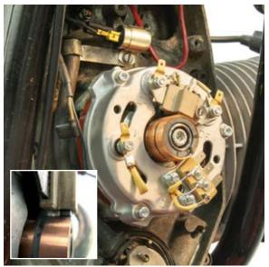
Secure the stator frame to the timing chain cover with the three mounting screws. Take care not to over tighten them and strip the aluminum timing chain cover. Insert the brush springs back onto the brushes and verify that the brushes align to their respective commutator ring only, and do not bridge the gap.
