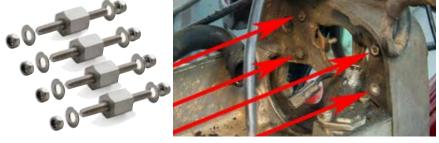
Connect the BLUE DF wire from the front engine harness to the DF terminal located on the back of the diode board. With this connection made, secure the diode board in place at the 4 mounting points on each corner with the M5x16 screws for early versions, or over the solid mounts securing the washer and nylock nuts, depending on your model.
