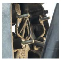
Later models with a 107mm stator use rubber mounts for the diode board. They can crack, dry, and fail causing the diode board to move and short. Equally, the diode board uses the mounting holes as its ground connection. With the rubber mounts, the grounding is done with ground wires. These brown ground wires can be reused or omitted at your discretion.
