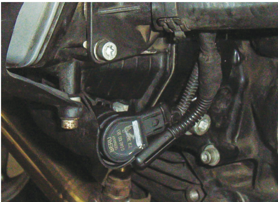
Left side coil cover and coil installed
