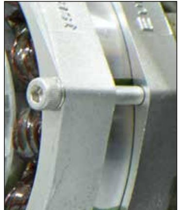
Fit the outer stator ring aligning the screw holes and secure the entire assembly with the bolts and lock washers included. Take great care not to over tighten as you can strip the threads on your aluminum engine. It may be easier to install the stator with both rings as one pre-assembled unit.
