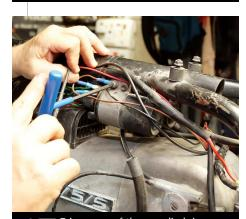
Crimp one of the supplied ring connectors to the brown ground wire from the module. We secured the ground wire at the front mount of the left coil, pairing it with factory ground wires already located there.
