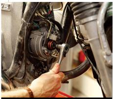
Next, remove the 6mm Allen head bolt securing the alternator rotor. It will usually break free with a sharp rap on a socket handle. If not, put the bike in gear and lock the rear brake.
