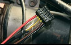
Following the manual instructions, install the wires as shown in the module plug and secure the clamping screws. From left to right: red ignition power supply wire; small white sensor unit wire; small yellow sensor unit wire; small brown sensor unit wire; brown ground wire; black negative coil wire.
