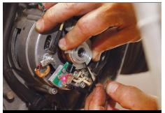
Set the engine at top dead center, "OT" on the flywheel. Reconnect the battery. Turn the ignition on. Loosen the trigger wheel. Rotate the trigger wheel clockwise until the red LED on the sensor lights. Continue slowly until the trigger wheel opening passes the sensor and just turns off the LED. Lock the trigger wheel set screws in place.
