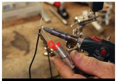
The kit includes three separate wires; brown wire for ground, black wire to ignition coil negative terminal, red wire to ignition positive power supply. With a soldering iron, tin one end of each wire. This ensures a positive connection when connected to the module plug.
