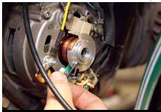
Start the engine. Using a timing light, check ignition timing at idle and full advance. We were spot on, requiring no further adjustment. Remove the trigger wheel set screws one at a time, coat with thread locking compound and reinstall. Disconnect the battery. Reinstall the front cover. Install the gas tank and reconnect the battery. Go ride.
