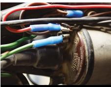
We needed an additional spade terminal on the positive side of the left coil for the red power lead to the module so we added a terminal from an old coil, then connected the red power lead after crimping on one of the supplied spade connectors.
