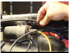
Since we left the points in place, we also left the wiring to the points in place. The points must be taken out of circuit, however, so we disconnected the points grounding lead at the right hand ignition coil, leaving the wire accessible.
