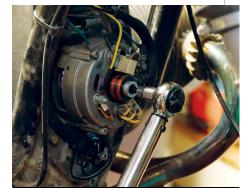
Lightly coat the bolt threads with thread locking compound. Install the bolt with the trigger wheel hub. Torque the bolt to 14ft/lb, slightly less than stock owing to reduced thread engagement due to the trigger wheel's thickness.
