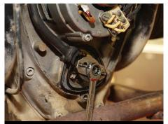
Remove the 10mm nut securing the mechanical advance unit. Remove the advance unit and replace the nut, being careful not to over-tighten it. You can leave the points in place as a backup; they'll no longer be actuated.
