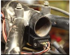
Using the included hook-and-loop material, mount the module under the rear of the top frame tube, toward the seat. Secure with the included zip ties. Plug the harness into the module and zip tie the wires together.
