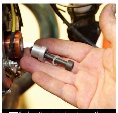
Replace the original washer on the alternator Allen bolt with the washer in the kit. Next, insert the bolt and washer through the trigger wheel hub.
