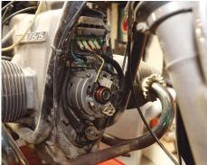
Disconnect the negative lead to the battery. Disconnect the fuel lines and remove the gas tank. Remove the three 5mm Allen head bolts securing the front cover, then remove the cover.
