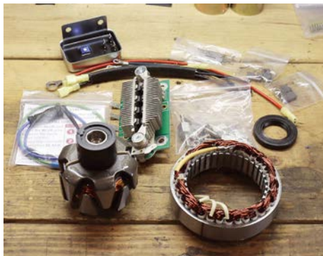
The upgrade kit includes a new 4-wire stator, rotor, diode board and mounts, regulator, brushes and wiring. The seal is optional.
