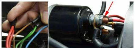
You will need to make a wire to connect the double red wire from the chassis harness to battery voltage. *It will match HAR-4B however needs a male spade terminal instead of female.* This wire runs from the **starter solenoid positive terminal**, to the **double red wire** from the chassis harness. This wire supplies voltage to power the bike.
