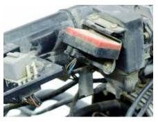
room for the R/R. Drill out the existing screw hole to the rear to accept the mounting bolt.
