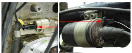
Run **HAR-4D** from the ignition **condenser** to the **coil negative** (terminal #1). This replaces the ignition wire removed that was part of the front engine harness.
