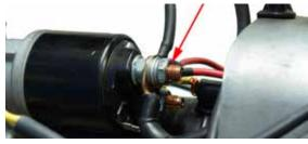
Connect the **BLACK** wire (with piggyback terminal) to the **coil positive** terminal. Use the piggyback to reconnect any wire (typically GREEN) that was removed to make
