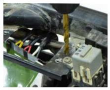
hardware. Note the R/R case is its ground connection, and for it to function properly and for its longevity, a solid ground connection is required. You may find it advantageous to install the additional ground strap included to ensure a proper ground connection.
