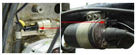
Run **HAR-4D** from the ignition **condenser** to the **coil negative** (terminal #1). This replaces the original ignition wire when you removed the front engine harness.
