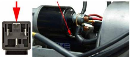
Run **HAR-4C** from the **starter solenoid spade terminal** to the new starter relay terminal **87**. This will trigger your starter to engage when you press your starter button.
