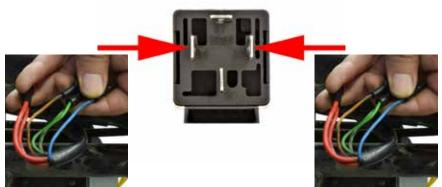
Connect the main harness **BROWN** to **86** and **GREEN** to **85** on the replacement relay.
