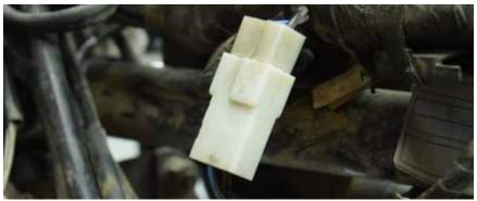
This connector can be problematic to disconnect. Take care when working with plastic connectors that are aged and brittle.
