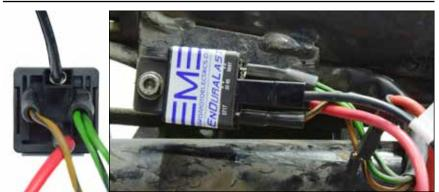
The relay will now look like this and can be secured with one of the original relay mounting screws to the frame as shown. **HAR-4A** will complete the remaining electrical connections as detailed below:
