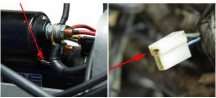
Run **HAR-4E** from the **starter solenoid spade terminal** to the **BLACK** wire in the plug as shown. This wire will trigger the starter when the start button is pressed and replaces the original wire removed with the engine harness.
