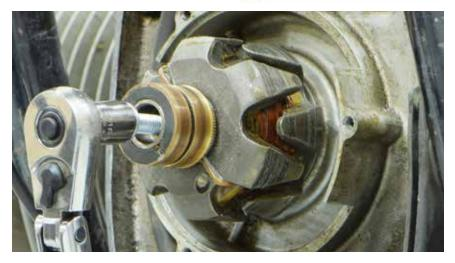
Gently tapping the rotor with a rubber mallet after tightening the removal tool can assist in releasing the rotor from the crankshaft. The rotor can "pop" off the end of the crankshaft, so be prepared! You may need to put the transmission in gear to keep the engine from turning over during this process.
