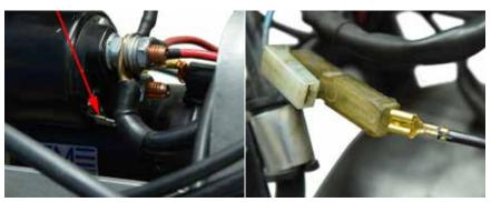
Run **HAR-4E** from the **Starter Solenoid Spade Terminal** to the **BLACK** wire in the white plug as shown. If your model does *not* have this plug, you will replace it with the bare connector into the relay block replacing the trigger wire for the starter. This wire will trigger the starter when the start button is pressed and replaces the original wire when you removed the engine harness.
