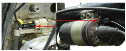
Run **HAR-4D** from the ignition **condenser** to the **coil negative** (terminal #1). This replaces the original ignition wire removed with the front engine harness.
