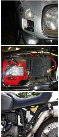
One location that is **NOT** recommended is **UNDER** the front engine cover, where the original diode board is located. Per the manufacturer (Ducati Energia) this R/R is not to exceed 194°F/ 90°C. The operating temperature here has been measured at 215°F/ 102°C. Do not cut or modify the R/R housing as it will more than likely cause damage.
