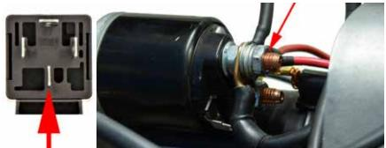
Run **HAR-4B** from the new starter relay terminal **30** to the **starter solenoid positive terminal**.
