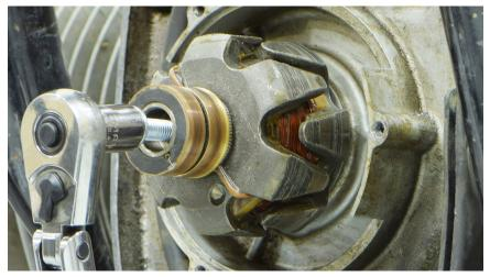
Gently tapping the rotor with a rubber mallet after tightening the removal tool can assist in releasing the rotor from the crankshaft. The rotor can "pop" off the end of the crankshaft, so be prepared!
