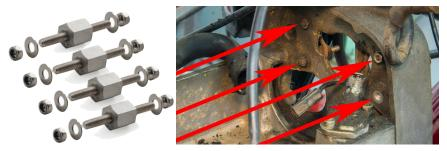
Connect the BLUE DF wire from the front engine harness to the DF terminal located on the back of the diode board. With this connection made, secure the diode board in place at the 4 mounting points on each corner with the M5x16 screws for early models, or over the solid mounts securing the washer and nylock nuts.
