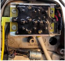
/5 and /6 models have a red wire as part of the front engine harness that connects to the starter relay from the diode board B+ terminal. Reconnect this wire as originally configured to the new diode board, that provides power to the bike. You can also run the included red wire as detailed below in addition to the original wire.
