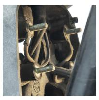
Later models with a 107mm stator use rubber mounts for the diode board. They can crack, dry, and fail causing the diode board to move and short. In addition, the diode board uses the mounting holes as its ground connection. With the rubber mounts, the grounding is done with ground wires. These brown ground wires can be reused or omitted at your discretion.
