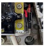
All models, will have wires to connect the brush holder as part of the front engine harness. Reconnect the brown to D- and blue to DF as marked on the stator frame cover.
