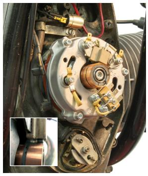
Secure the stator frame to the timing chain cover with the three mounting screws. Take care not to over tighten them and risk striping the aluminum timing chain cover.
