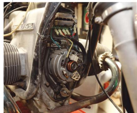
**1** Disconnect the negative lead to the battery. Disconnect the fuel lines and remove the gas tank. Remove the three 5mm Allen head bolts securing the front cover, then remove the cover.
