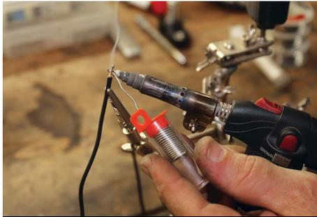
**11** The kit includes three separate wires; brown wire for ground, black wire to ignition coil negative terminal, red wire to ignition positive power supply. With a soldering iron, tin one end of each wire. This ensures a positive connection when connected to the module plug.
