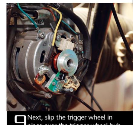
**9** Next, slip the trigger wheel in place over the trigger wheel hub, centering the disc in the black sensor pickup slot. Lightly tighten the two small Allen head screws to secure the trigger wheel. The exact position of the trigger wheel will be set later.
