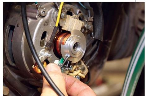
**18** Start the engine. Using a timing light, check ignition timing at idle and full advance. We were spot on, requiring no further adjustment. Remove the trigger wheel set screws one at a time, coat with thread locking compound and reinstall. Disconnect the battery. Reinstall the front cover. Install the gas tank and reconnect the battery. Go ride.
