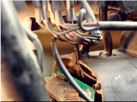
**10** Route the sensor harness to and through the top of the front cover. We cut a small relief in the grommet for the charging wires, making sure the sensor harness wouldn't be crimped by the cover once installed.
