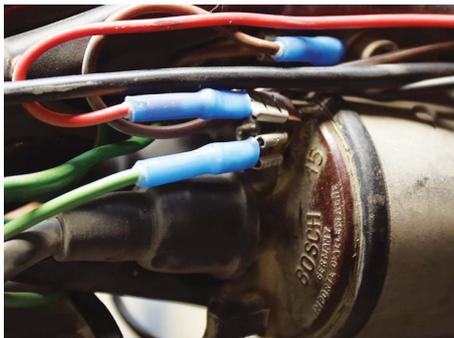
**14** We needed an additional spade terminal on the positive side of the left coil for the red power lead to the module so we added a terminal from an old coil, then connected the red power lead after crimping on one of the supplied spade connectors.
