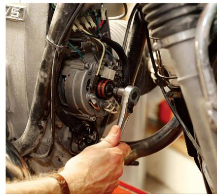
**4** Next, remove the 6mm Allen head bolt securing the alternator rotor. It will usually break free with a sharp rap on a socket handle. If not, put the bike in gear and lock the rear brake.
