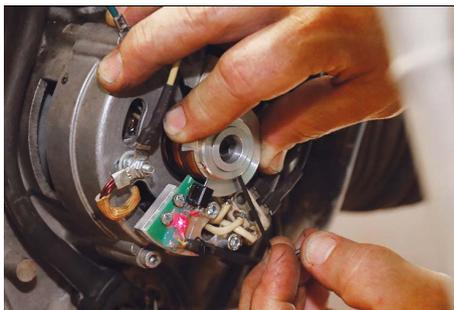
**17** Set the engine at top dead center, "OT" on the flywheel. Reconnect the battery. Turn the ignition on. Loosen the trigger wheel. Rotate the trigger wheel clockwise until the red LED on the sensor lights. Continue slowly until the trigger wheel opening passes the sensor and just turns off the LED. Lock the trigger wheel set screws in place.
