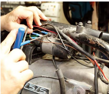
**16** Crimp one of the supplied ring connectors to the brown ground wire from the module. We secured the ground wire at the front mount of the left coil, pairing it with factory ground wires already located there.
