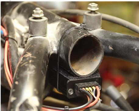
**13** Using the included hook-and-loop material, mount the module under the rear of the top frame tube, toward the seat. Secure with the included zip ties. Plug the harness into the module and zip tie the wires together.
