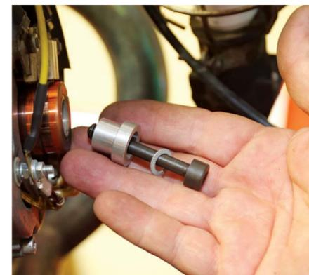
**5** Replace the original washer on the alternator Allen bolt with the washer in the kit. Next, insert the bolt and washer through the trigger wheel hub.
